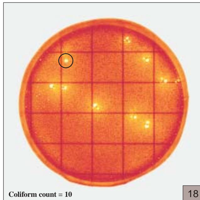
A dilution of chocolate is shown in figure 18. Zones of acid associated with colonies will continue to expand during incubation. Gas bubbles associated with colonies are another criteria that will aid in the identification of coliforms. Gas bubbles may outline the colony as shown in the circle. Enumeration with or without gas is method dependent.
