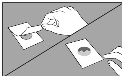
**9** Carefully **ROLL** top film down to avoid entrapping air bubbles. **Do NOT** let top film drop.
