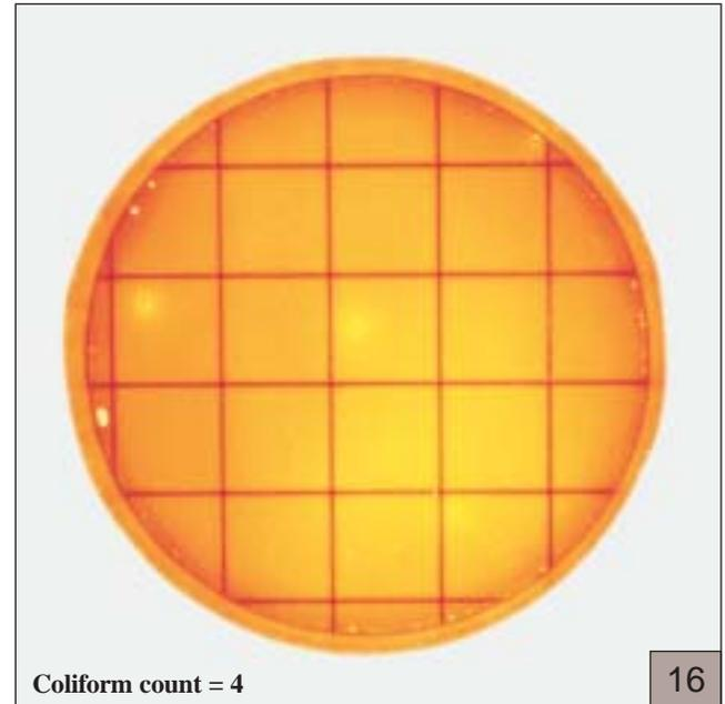
Despite the change in gel color, acid produced by the coliforms is still easily seen, as shown in figure 16.
