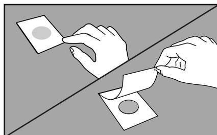
**7** Place Petrifilm plate on **level** surface. Lift top film.
