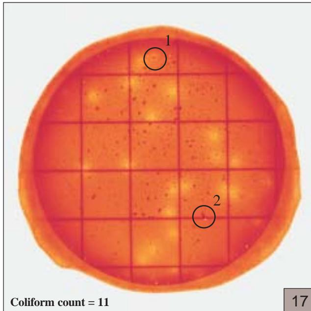
Figure 17 is an early reading of a dilution of paprika. Circle 1 shows an acid zone around a red, irregularly-shaped food particle. Some foods may contain acidic particles that react with the pH indicator. Circle 2 shows a bubble near a red, irregularly-shaped food particle—but no acid zone. Neither should be counted as a colony.
