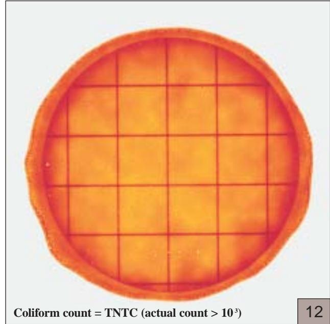
The Petrefilm RCC plate in figure 12 has two characteristics indicating TNTC colonies: change in gel color and many small colonies.
