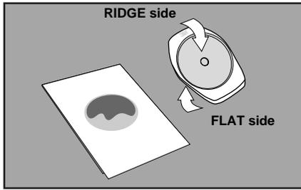
**10** With **FLAT** side down, place spreader on top film over inoculum.
