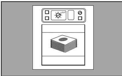
**13** Incubate plates with clear side up in stacks of up to 20 at a temperature of  $35^{\circ}\pm 1^{\circ}\text{C}^*$  for up to  $24 \pm 2$  hours, examining plates at timed intervals depending on desired information (refer to package insert).
