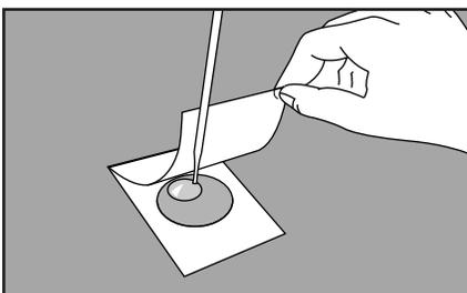
**8** With pipette **perpendicular** to Petrifilm plate, place 1 mL of sample onto center of bottom film.
