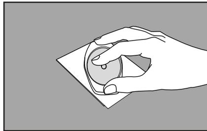
**11** **GENTLY** apply pressure on spreader to distribute inoculum over circular area. Do not twist or slide the spreader.
