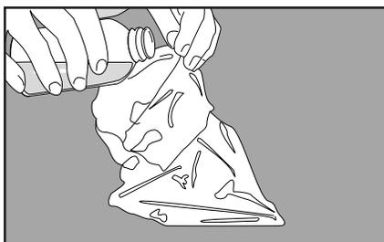
**5** Add appropriate quantity of one of the following sterile diluents: Butterfield's phosphate buffer (IDF phosphate buffer, 0.0425 g/L of  $\text{KH}_2\text{PO}_4$ , adjusted to pH 7.2), 0.1% peptone water, peptone salt diluent (ISO method 6887), saline solution (0.85 - 0.90%), or distilled water.
