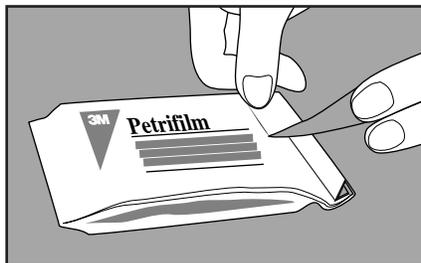
**2** To seal opened package, fold end over and tape shut.
