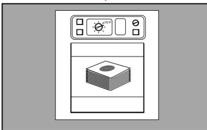
**13** Incubate plates with clear side up in stacks of up to 20 at a temperature of  $35 \pm 1^\circ\text{C}^*$  for up to  $24 \pm 2$  hours, examining plates at timed intervals depending on desired information (refer to package insert).
