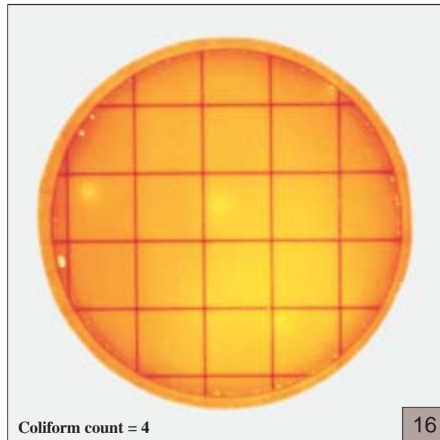
Despite the change in gel color, acid produced by the coliforms is still easily seen, as shown in figure 16.
