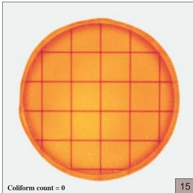
Compare the negative plate above to the TNTC plates on the previous page. Note that no colonies or gas bubbles are present in figure 15 to indicate a TNTC result.
