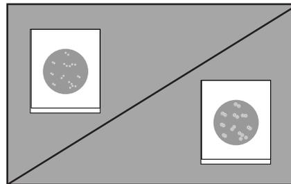
**14** Read Petrifilm plates using indirect light for early detection. Petrifilm plates can be counted on a standard colony counter or other magnified light source. Refer to the *Interpretation Guide* section when reading results.
