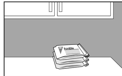
**3** Keep resealed package at  $\leq 25^{\circ}\text{C}$  ( $\leq 77^{\circ}\text{F}$ ) and  $\leq 50\% \text{RH}$ . **Do not refrigerate opened packages.** Use Petrifilm plates within one month after opening.
