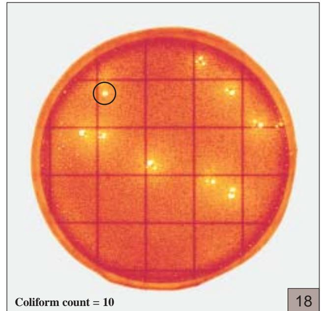
A dilution of chocolate is shown in figure 18. Zones of acid associated with colonies will continue to expand during incubation. Gas bubbles associated with colonies are another criteria that will aid in the identification of coliforms. Gas bubbles may outline the colony as shown in the circle. Enumeration with or without gas is method dependent.
