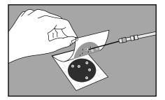
17 If further identification is desired, lift top film and pick the colony from the gel.
