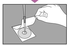
Place Petrifilm Plate on level surface. Lift top film. With 3M™ Electronic Pipettor or equivalent held perpendicular to Petrifilm Plate, place 1 mL of sample or diluted sample onto center of bottom film.
