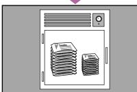
Store unopened pouches of plates and disks at  $\leq 8^{\circ}$  C ( $\leq 46^{\circ}$  F). Use before expiration date on package. In areas of high humidity where condensate may be an issue, it is best to allow pouches to reach room temperature before opening.
