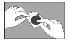
14 Apply gentle pressure to the disk area, including the edges of the disk, by sliding a finger firmly across the top film. This will ensure uniform contact of the disk with the gel and will eliminate any air bubbles.
