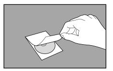
8 ROLL top film down onto sample gently to prevent pushing sample off film and to avoid entrapping air bubbles. Do not let top film drop.
