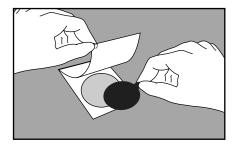
13 Remove a disk from its individual package by grasping the tab. Lift the top film of the Petrifilm Plate and place the disk in the well of the plate. Lower the top film.
